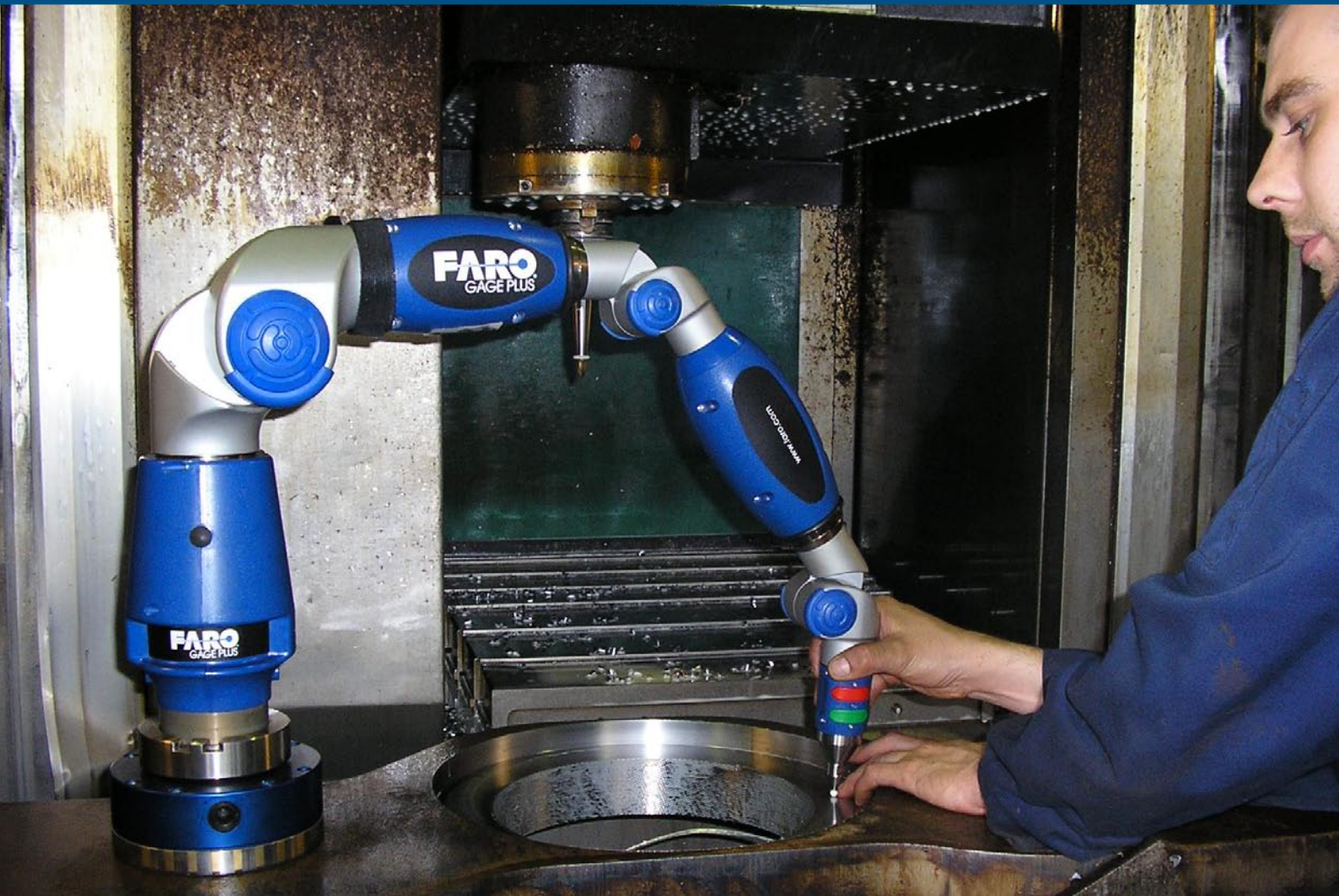
Production areas included verification of components on machine.
