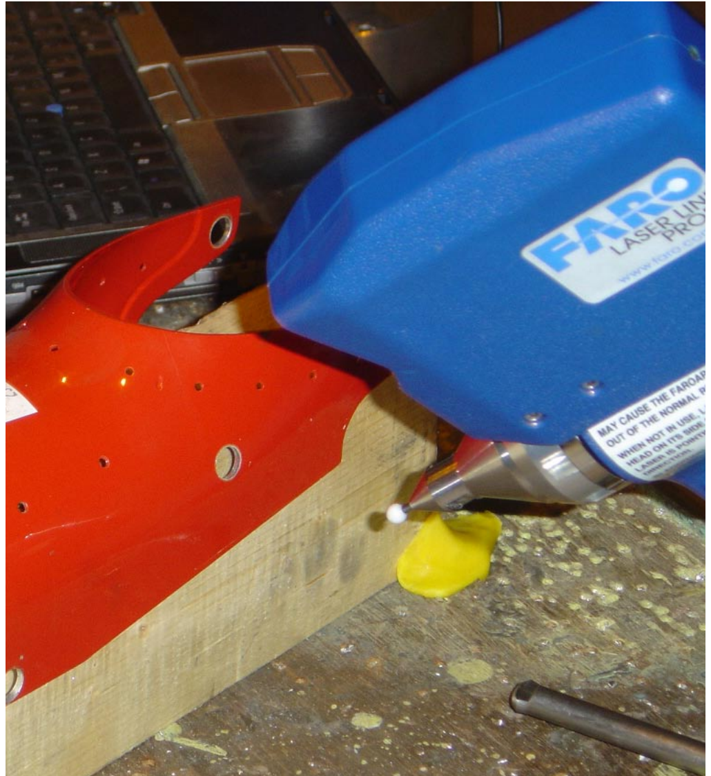
The ScanArm measures at a speed rate of more than 19,000 points per second.
